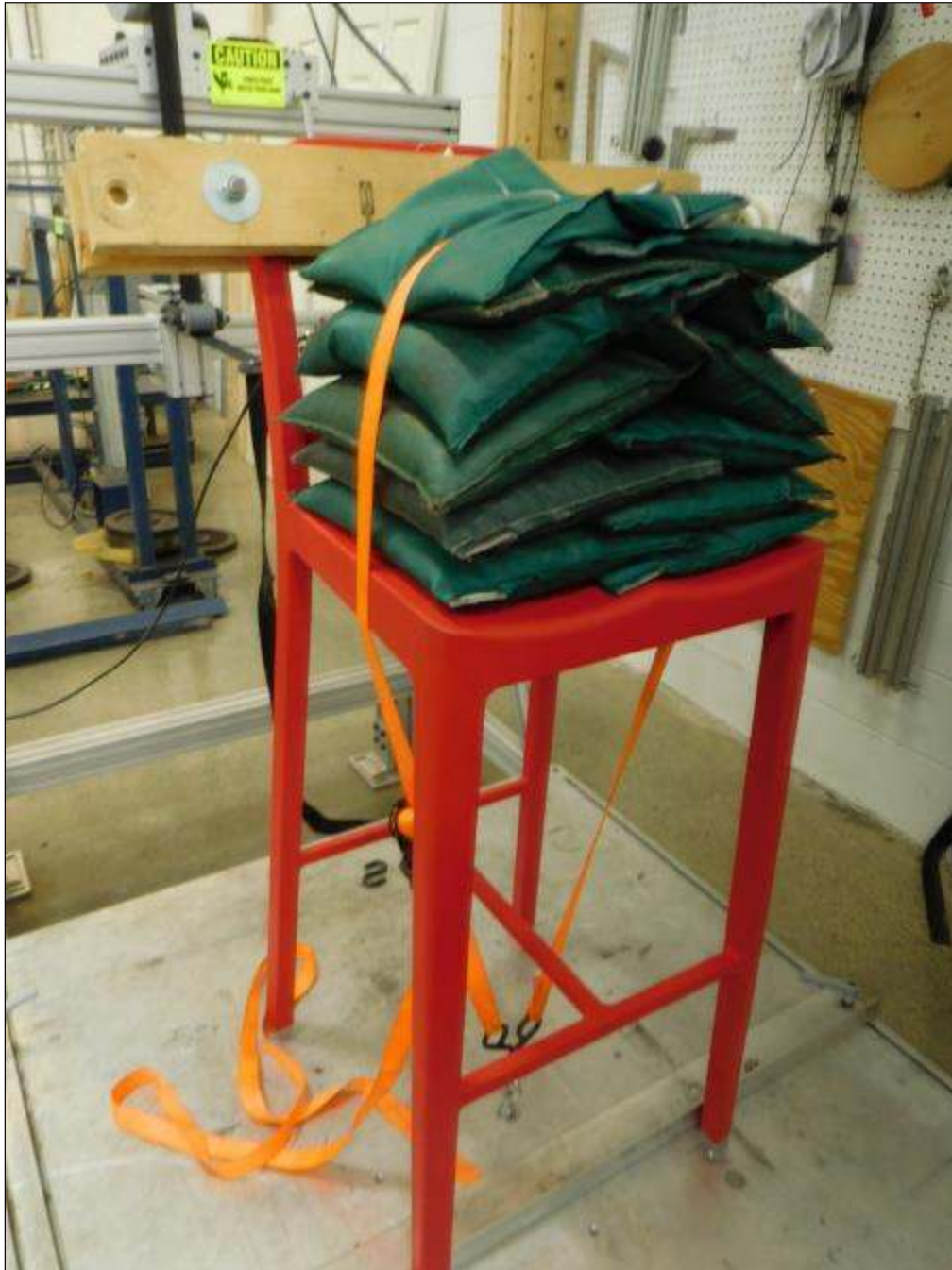
Backrest Durability Test – Cyclic
