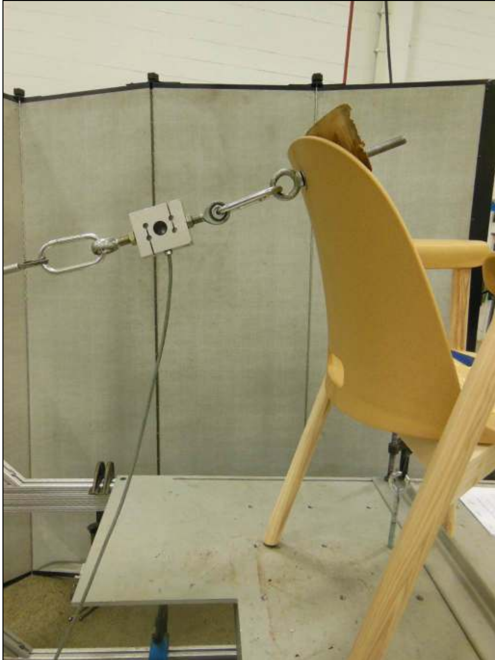
BACK STRENGTH PROCEDURE - STATIC
