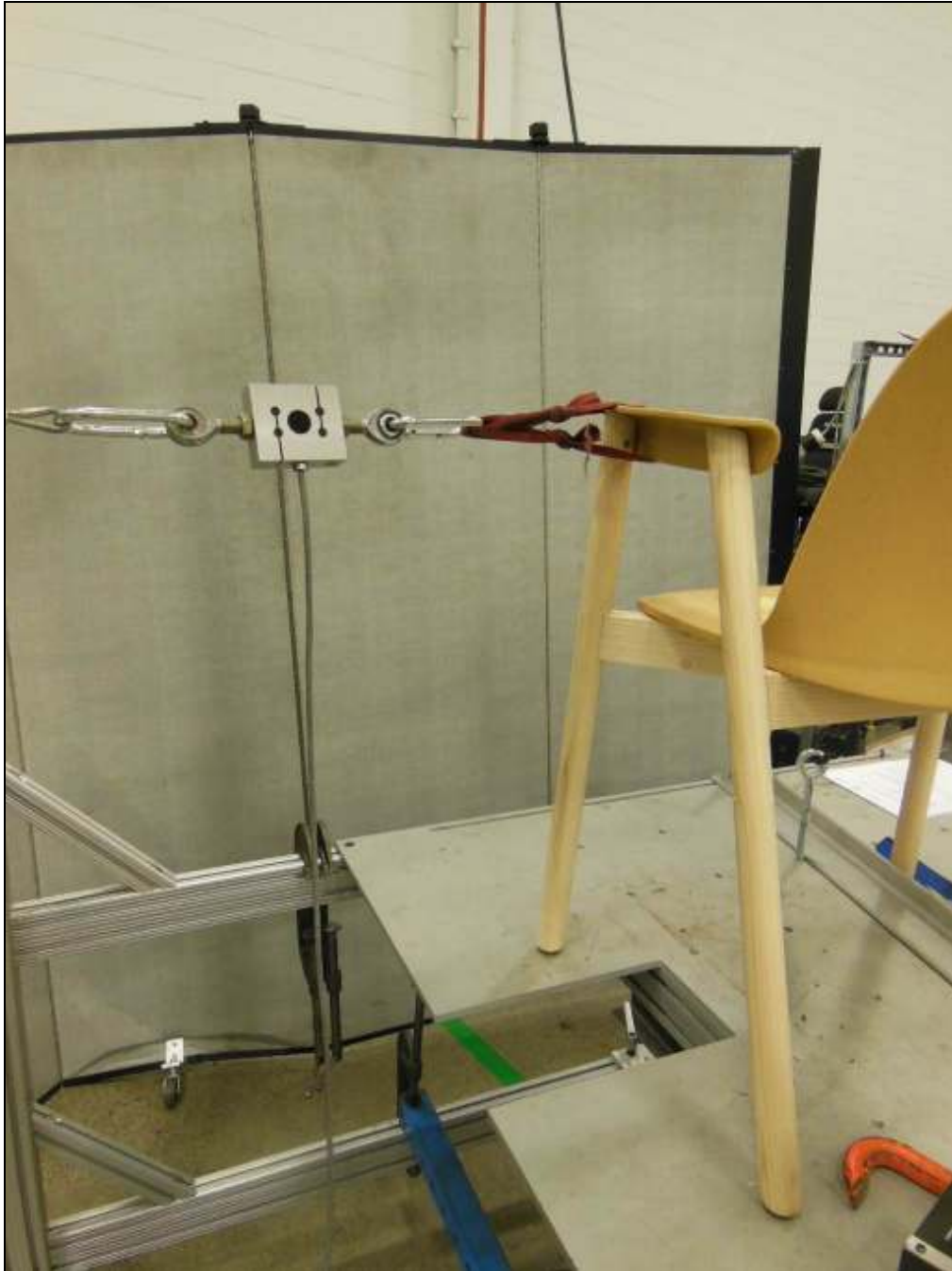
Arm Strength Test- Horizontal-Static
