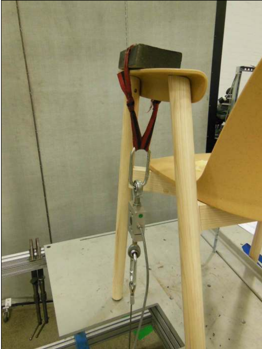
Arm Strength Test Vertical-Static
