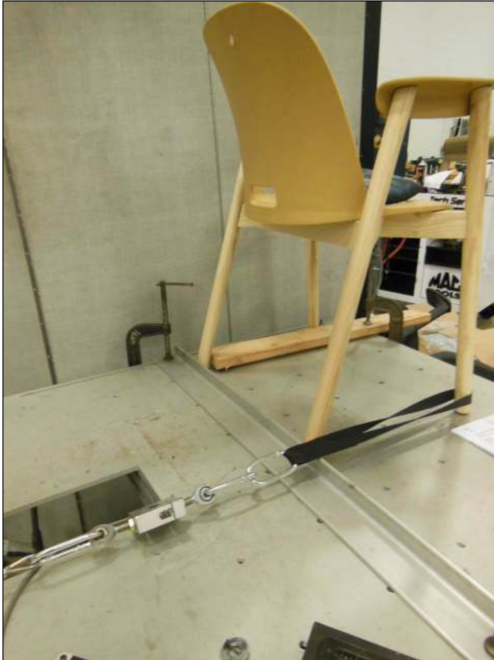
LEG STRENGTH TEST - FRONT APPLICATION
