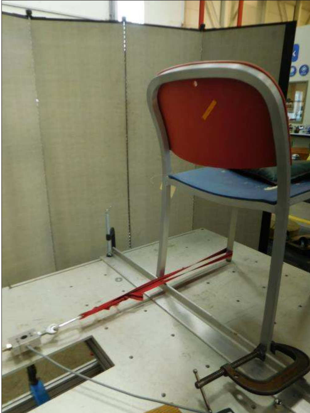
Leg Strength Test – Front Load
