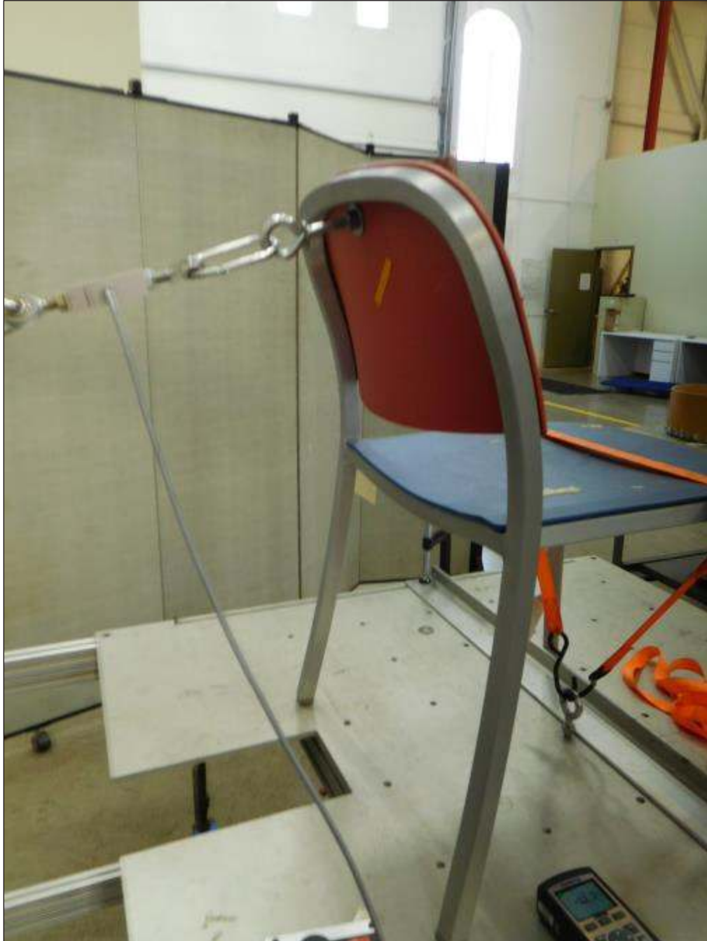
Backrest Strength Test – Static
