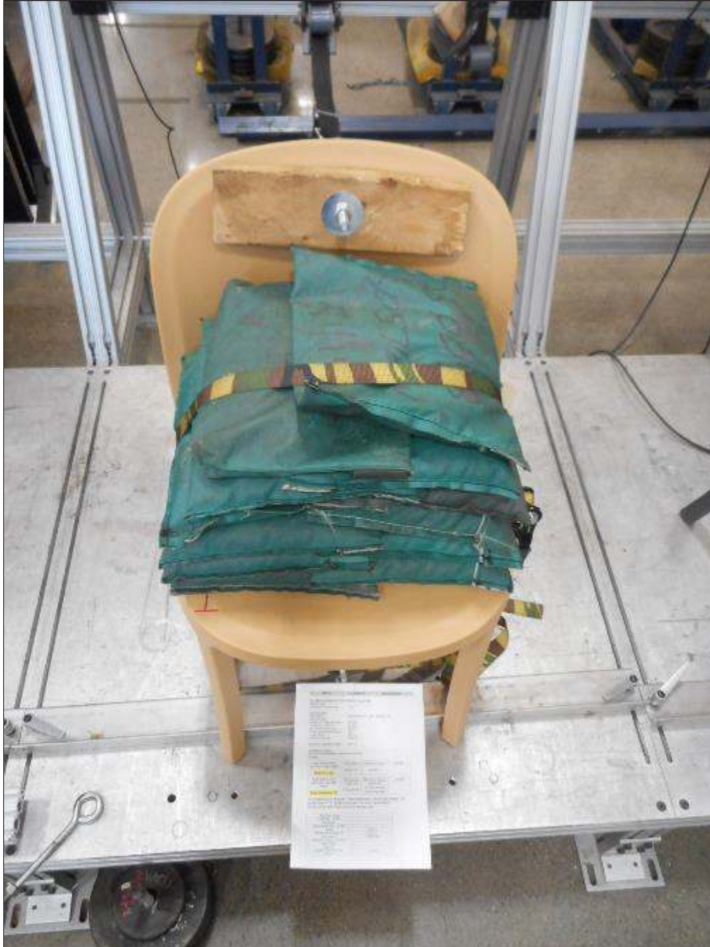
Backrest Durability Test – Cyclic
