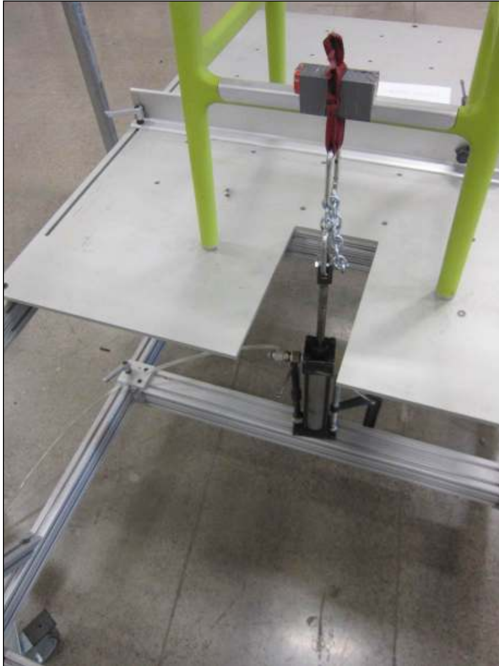
FOOTREST STATIC LOAD TEST – GREEN
