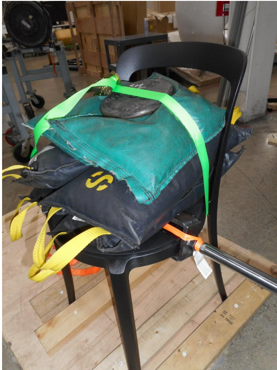
Structural Durability Test – Cyclic - Side to Side
