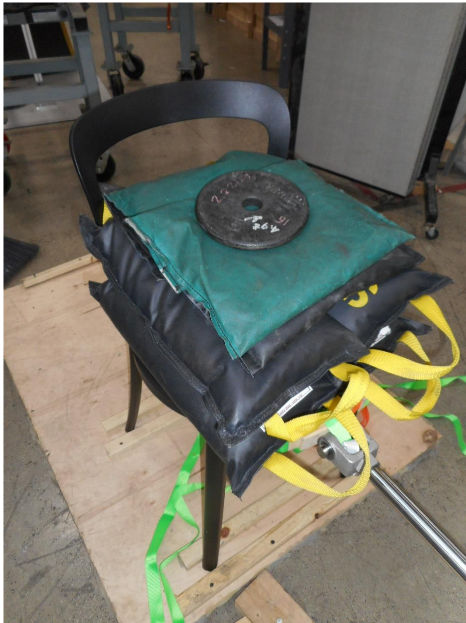
Structural Durability Test – Cyclic - Front to Back
