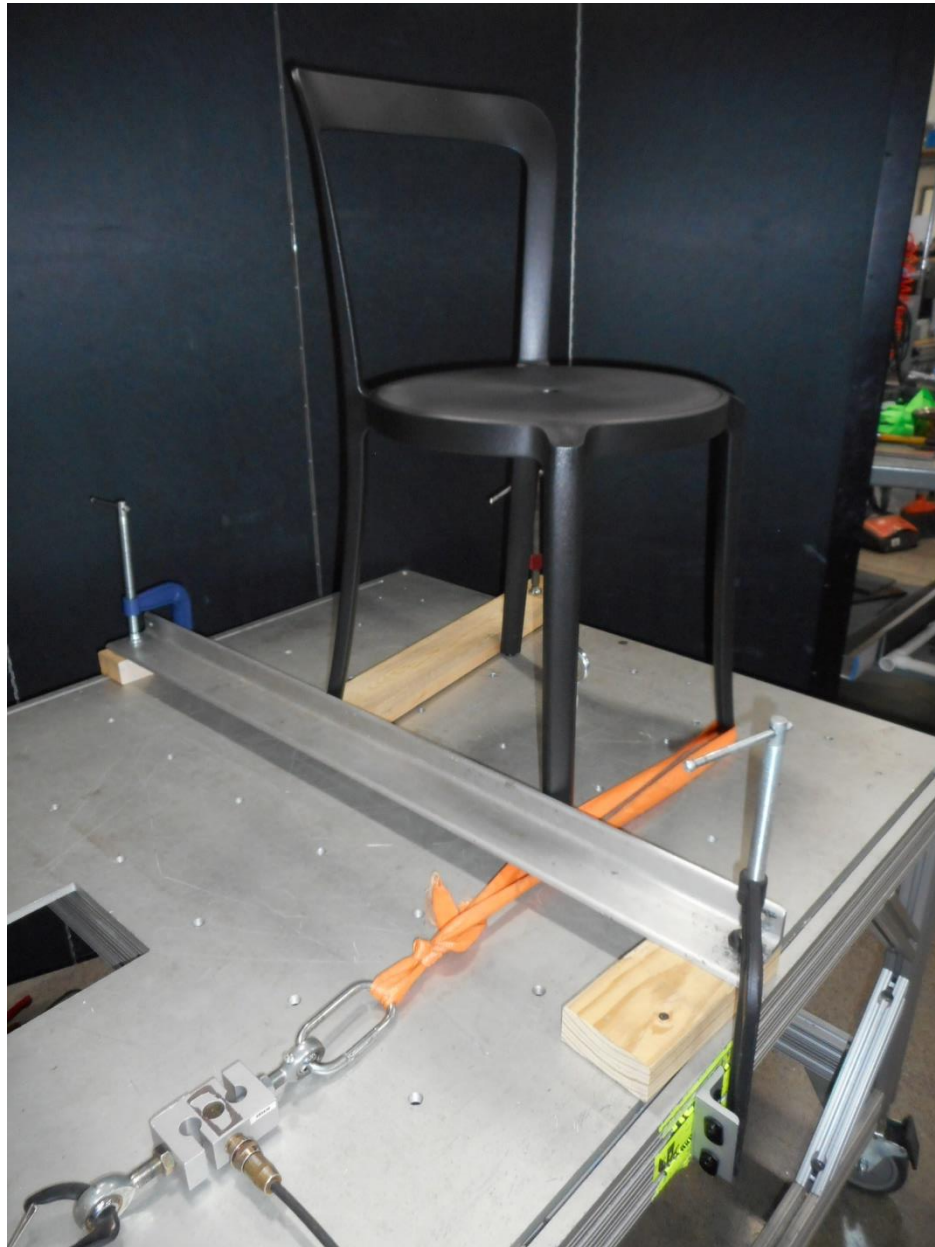
Leg Strength Test – Side Load
