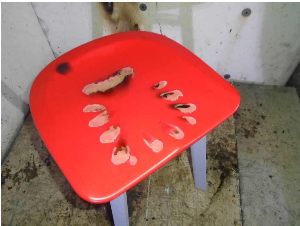
SU STOOL - RECYCLED POLYETHYLENE - Post-Test
