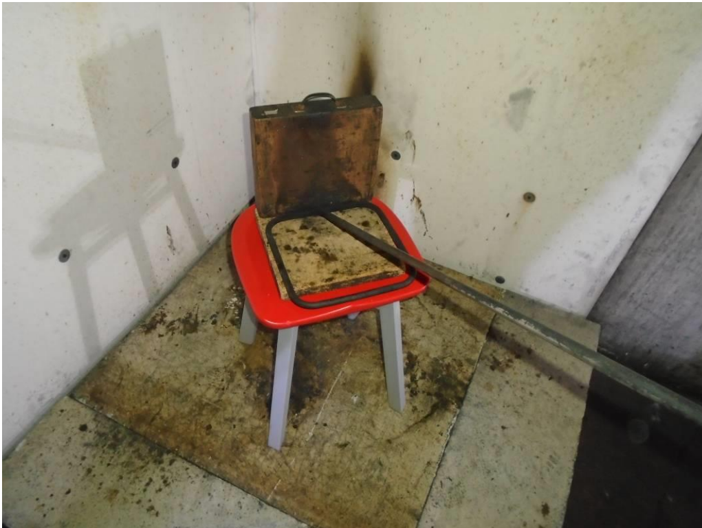
SU STOOL - RECYCLED POLYETHYLENE - Pre-Test Setup
